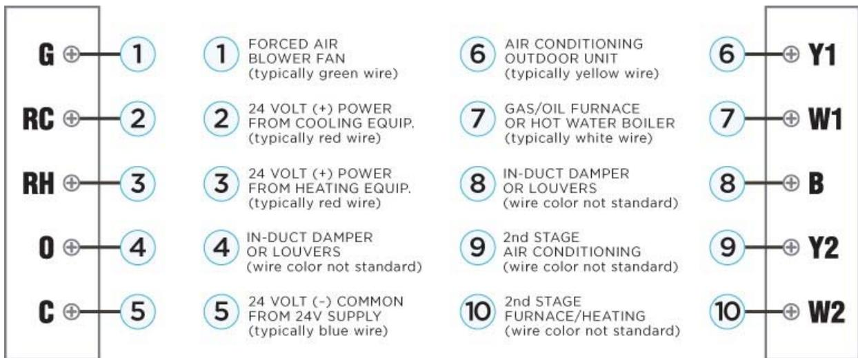
If you have separate RH and RC wires, please remove the RED RC-RH shorting cap from the back of the thermostat.
